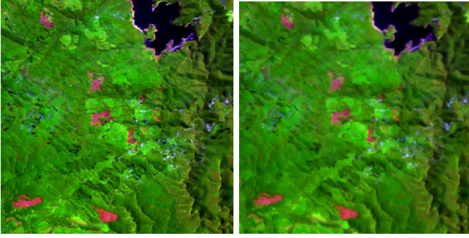
Fig. 6: Left : Gap filling output, Right : The masked sparse reconstruction step reduces noise and removes boundary effects caused by the gap filling.
